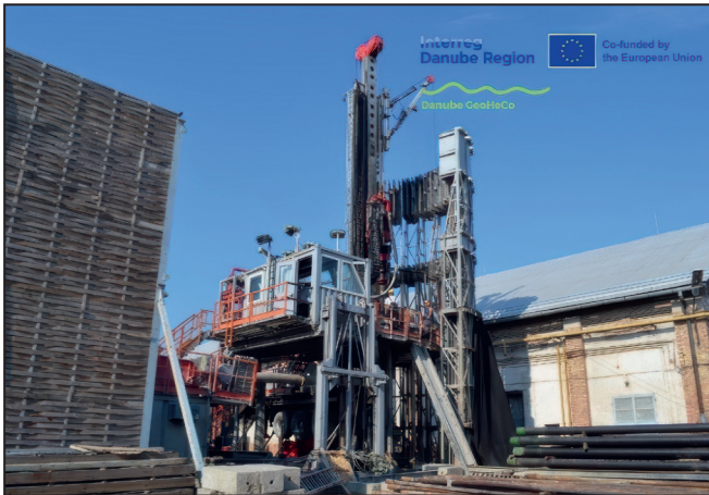
Directional well drilling; Photo by InnoGeo Research and Service Ltd.
