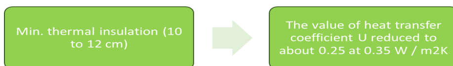
Figure 2.1 The value of heat transfer reduction after applying 10 to 12 cm of thermal insulation
