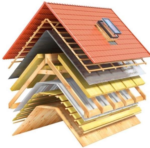
Figure 4. Thermal insulation of roof 4
